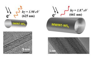
With different electro-optical properties than their bulk counterparts, interest in nanotubes has exploded. Initially, nanotubes were built from carbon, but researchers are increasingly exploring other inorganic materials. Ghosh et al. studied the electro-optical behavior of single wall tungsten disulfide nanotubes for the first time and discovered interesting new luminescent properties.
